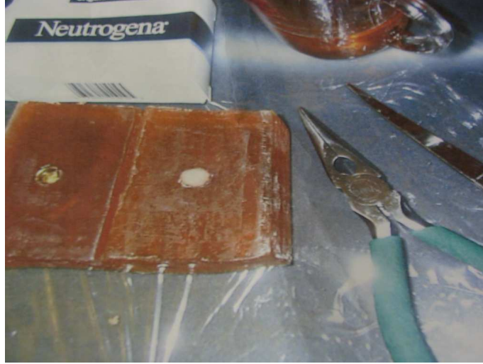
Figure 44.: Sliced MREIM phantom constructed of fragrance free Neutrogena soap showing the spherical piece of fat-free hotdog of 1 cm in diameter (cancer surrogate).
