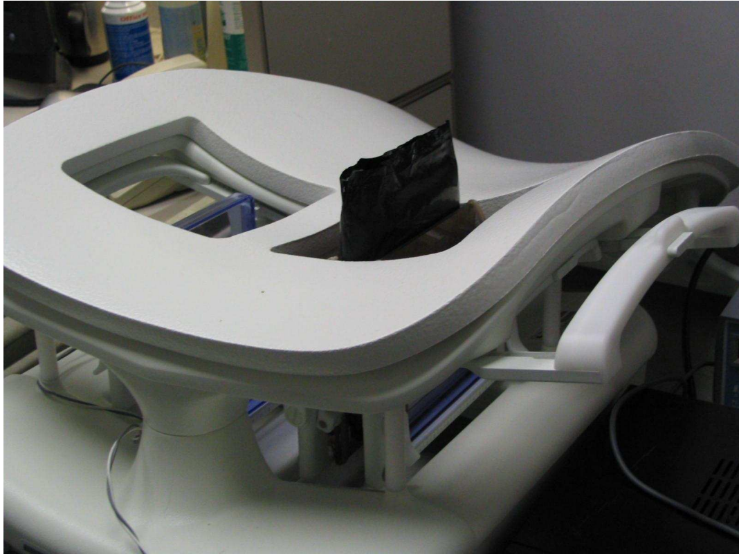
Figure 50.: A Siemens 1.5 T Symphony 7 Channel Biopsy Breast Array provided by Invivo Corp. (Orlando, FL) with the stabilization paddles modified to include the Faraday shield electrodes.
