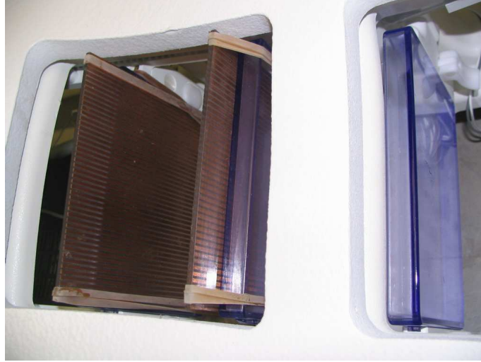
Figure 51.: Stabilization/compression paddles of the MR breast coil. The left paddle of the coil was modified to include a Faraday shield made of a pair of copper sheets consisting of rectangular parallel bars. The copper sheets shown here had dimensions of 14 \times 15 \text{ cm}^2 . The phantoms were positioned between the two plates for imaging.
